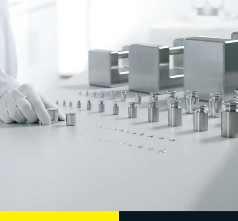
OIML class F1 and F2 cylindrical weights with a lug are made of a special stainless steel that has a density of 7,950 kg/m³, and their tolerances comply with OIML R111-1. The weights are delivered in a wooden case suitable for transportation by a pallet mover.
